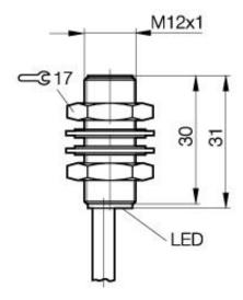
Inductive Sensors BES 516-370-E4-Y M12x1 x 31 normally-closed Sn=2mm shielded
